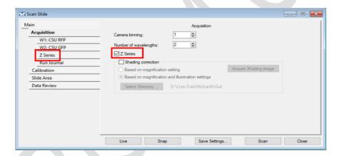
(5) Click on "Z Series" tab to open Z series window. Choose "range around current" to define range and step size or uncheck to define top and bottom.
