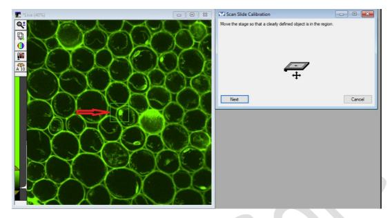
4. Move stage so the clear object is in the center of the purple frame.
