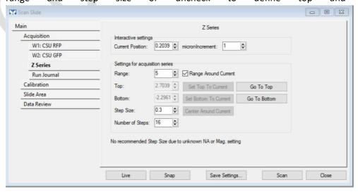
(6) By default, the system uses Piezo Z motor for Z series acquisition, which requires user to use the small up and down arrow to move the stage up and down, not the focus knob on the microscope.
