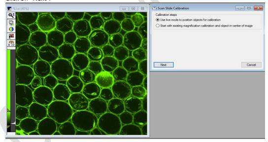
3. Identify a clear object and move the stage so the object is in the center of the green frame.
