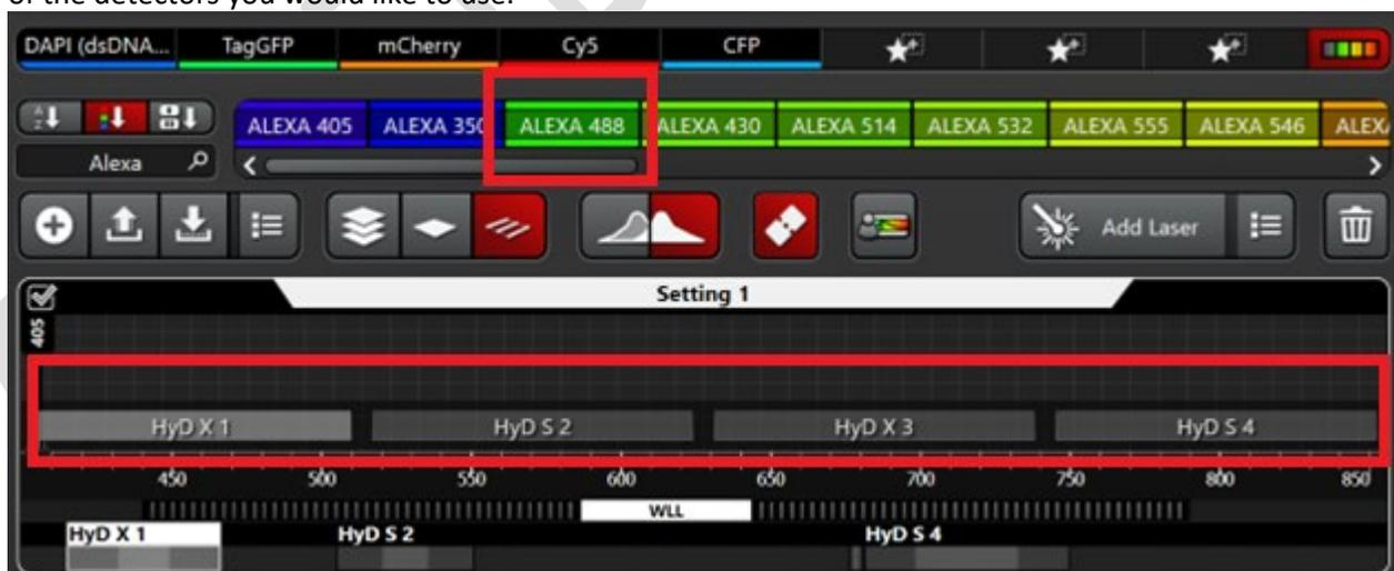
4. Once the detector is linked, e.g. HyD S2 as shown on the picture below. Select the detector, turn it on and select the “Counting” for “operating mode”, of which the grey value of pixels are the photon numbers. “Analog” is the normal mode for most confocal instruments.
