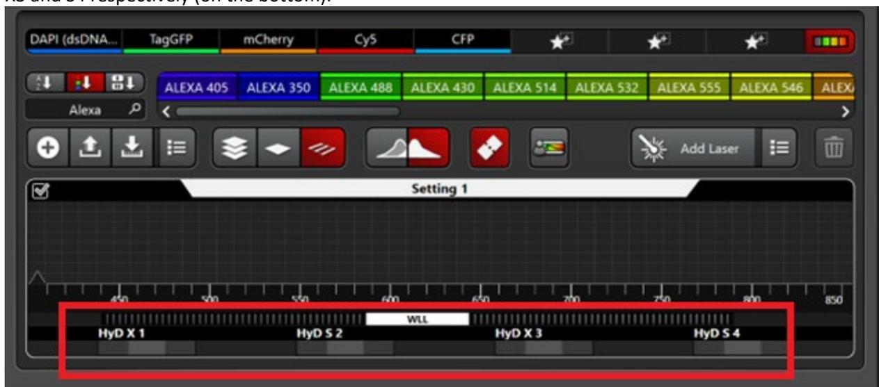
3. Find labels icon (e.g. Alex488, as shown on the picture below) and drag it onto the “setting” field, while the four detector icons automatically appear onto the field too. Drop the label icon into one of the detectors you would like to use.
